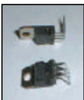
Legs bent on regulators
