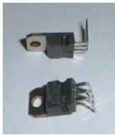
Legs bent on regulators
